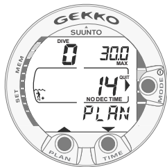
Fig. 3.5. Dive Planning. Planning mode is indicated by PLAN text. No-decompression time limit at 30.0 m [100 ft] is 14 minutes in A0/P1 mode.
