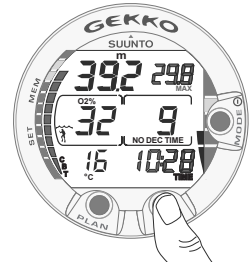
Fig. 3.24. Alternative display. Pressing TIME button displays current time, maximum depth, temperature, CBT and O_2\% ,
