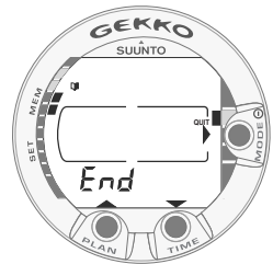
Fig. 4.11. Logbook, end of the memory. END text is displayed between oldest and the most recent dive.
