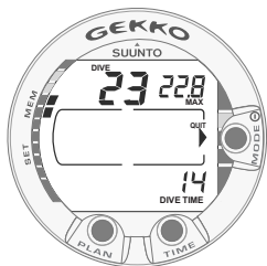
Fig. 4.13. Dive History information. Total number of dives, dive hours and maximum depth.
