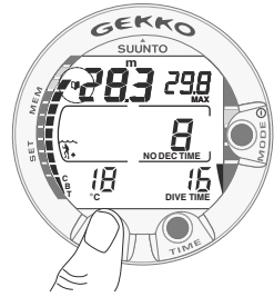
Fig. 3.8. Bookmark activation. An annotation, Bookmark, is placed in the profile memory during a dive by pressing PLAN button. Note Logbook symbol.
