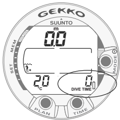
Fig. 3.4. Low Battery Warning. Battery symbol indicates that the battery is low and battery replacement is recommended.
