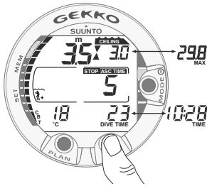
Fig. 3.17. Decompression dive, at ceiling zone. Two arrows point at each other (“hour glass”). You are in the optimum ceiling zone at 3.5 m [11 ft] and your minimum ascent time is 5 minutes. Pressing TIME button activates alternative display.
