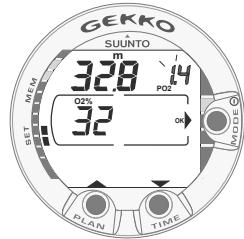
Fig. 4.17. Setting Nitrox parameters, Oxygen percentage is 32%, oxygen partial pressure limit is 1.4 bar. The equivalent maximum depth is displayed as 32.8 m [107 ft]. Press scroll buttons to change oxygen percentage and to set oxygen partial setting value. Accept settings by pressing MODE (OK).
