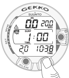
Fig 3.27. Surface interval, Surface time display. Pressing TIME button once will show surface time display.
