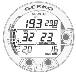
Fig. 3.25. The lowest bar graph blinks to indicate that the OLF value shown relates to OTU.
